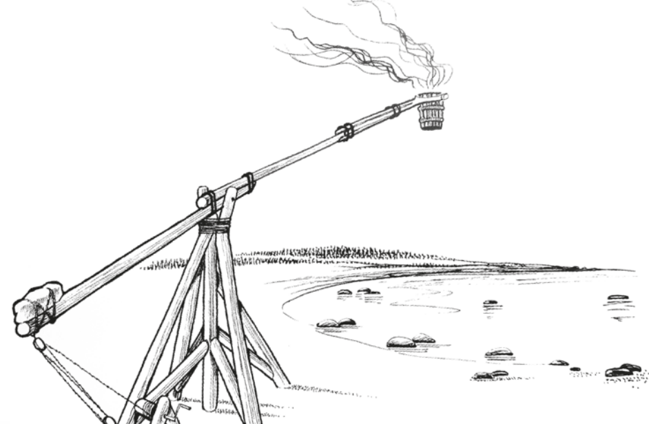
Lever lights (Danish: vipp-fyr ) were invented in Denmark in 1626, drawing by R. Matkiewicz.
