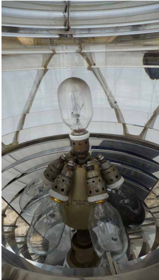
EMN-500 light system bulb changer in Fresnel dioptric lens, photo by V. Laitus
